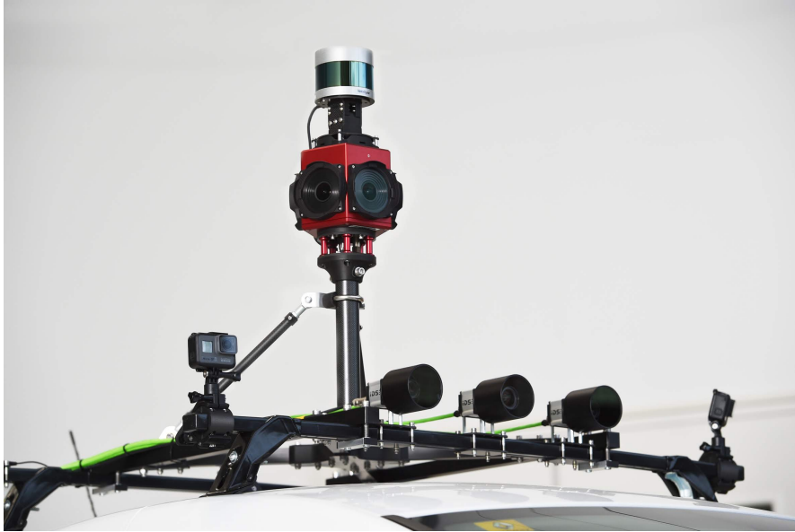
Figure 1: A typical sensor suite on top of a car, with multiple cameras and LIDAR sensors. Photo from QUT.
