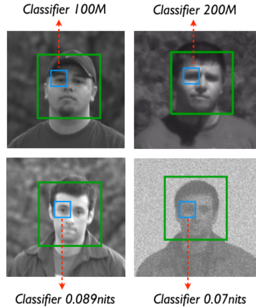
Fig. 1 The approach: build classifiers for different conditions, such as distance and illumination. While general enough for any feature that can be represented by a window of pixels, the eye is shown here, and in subsequent figures, as an example
